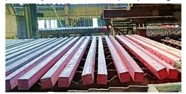
is converter slag.In the steel casting ladle, the steel undergoes out-of-furnace processing before being sent to the continuous casting machine section. Here, the steel is crystallized, formed, cooled, and labeled. The final product is a concast steel billet.The continuous cast billet is manufactured according to approved technological instructions. The raw material for billet production is steel of various grades. The steel grade for billet production
